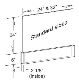
Dimension 'C' should be the precise thickness of your divider. We will add 1/8" to ensure that the shield fits and will slip down into place on the divider.
